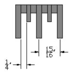
Ultra close-mesh Peds & Treads Heavy Duty Bar Grating with 1/4" opening is specially designed for street and sidewalk applications where pedestrians in high heels, bicycles and wheel chairs must be accommodated while providing load carrying capacity for truck traffic.
