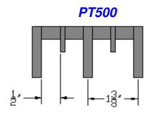
Peds & Treads Heavy Duty Bar Grating with 1/2" opening is specially designed for street and sidewalk applications where the "Americans with Disabilities Act" applies and truck traffic is present.
